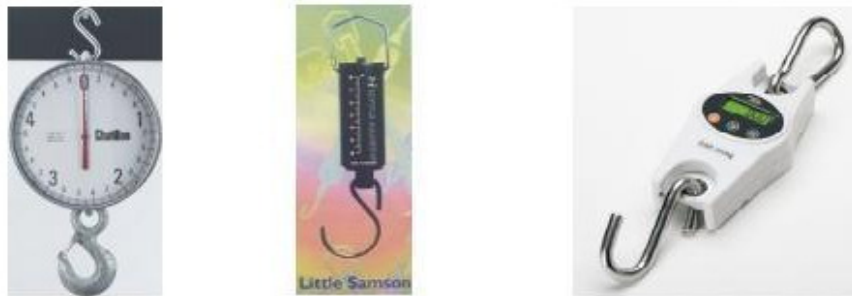
Gambar 4.1 Berbagai macam neraca pegas http://ybap.wordpress.com/2011/09/26/beberapa-alat-praktikum-fisika-1/
