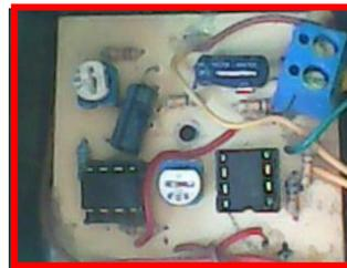
PCB Sistem Minimum ATmega8 Sesudah Pelarutan
