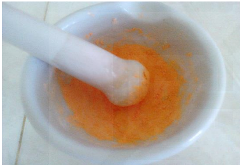
Proses penggerusan reagen (asetofenon, NaOH dan vanilin)
