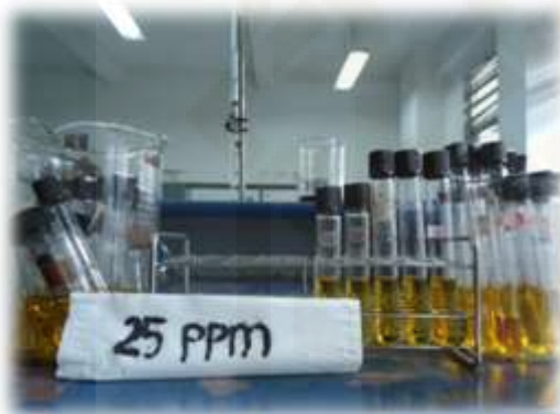
Gambar 5.40 Uji COD sampel-limbah tapioka ( KMnO_4 25 ppm)
