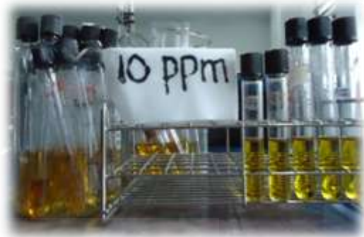
Gambar 5.39 Uji COD sampel-limbah tapioka ( KMnO_4 10 ppm)
