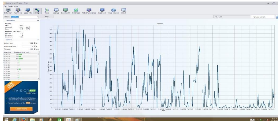
Gambar 1.67 Packet Loss gedung lantai 2 pukul 12:45 – 15:30
