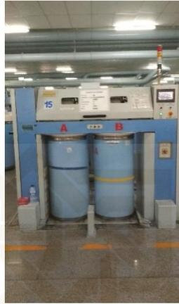
**Gambar 4.5. Drawing Breaker spinning X**
