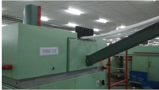
**Gambar 4.6. Drawing Finisher spinning X**
