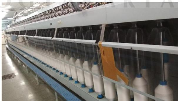
**Gambar 4.7. Speed Frame spinning X**
