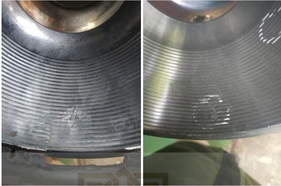
Gambar Tampak Cacat Coldshuts Downlight
