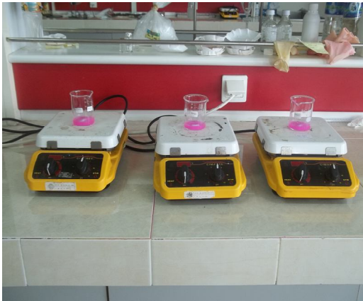
Gambar 3. Proses adsorpsi zeolit terhadap rhodamin B
